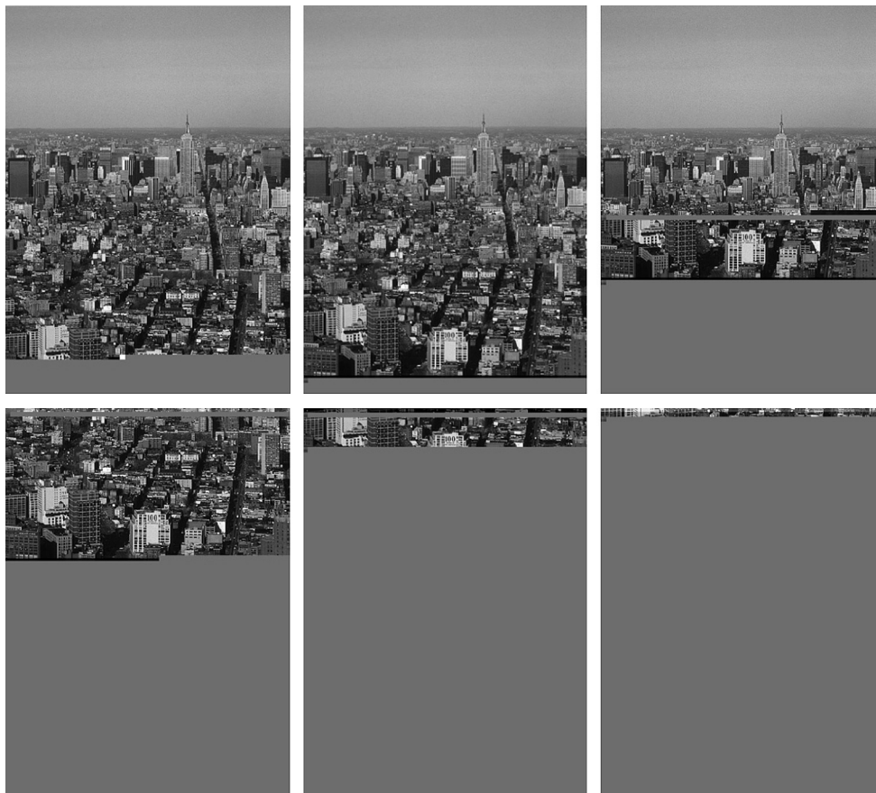
Fig. 5 – Recovered files after erasure of random amounts of data from tail (upper left), center (upper center and right), and both header and tail parts (lower row) of the original image.
