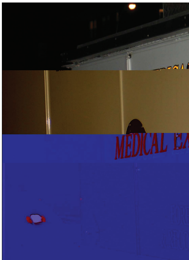
[FIG9] Fully validated but incorrect JPEG image from the DFRWS 2007 test set.
